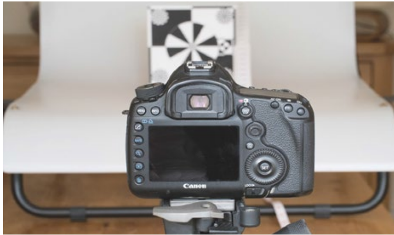
Many DSLRs allow you to calibrate the autofocus response
